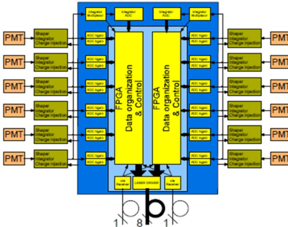
Scheme for 12-PMT MainBoard
