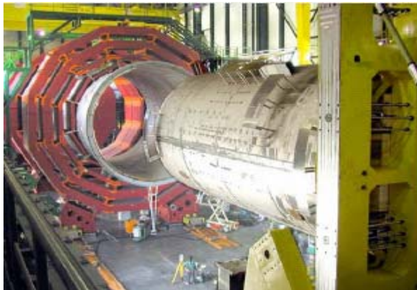
Muon Spectrometer ( |\eta| < 2.7 ) • air-core toroids with muon chambers
